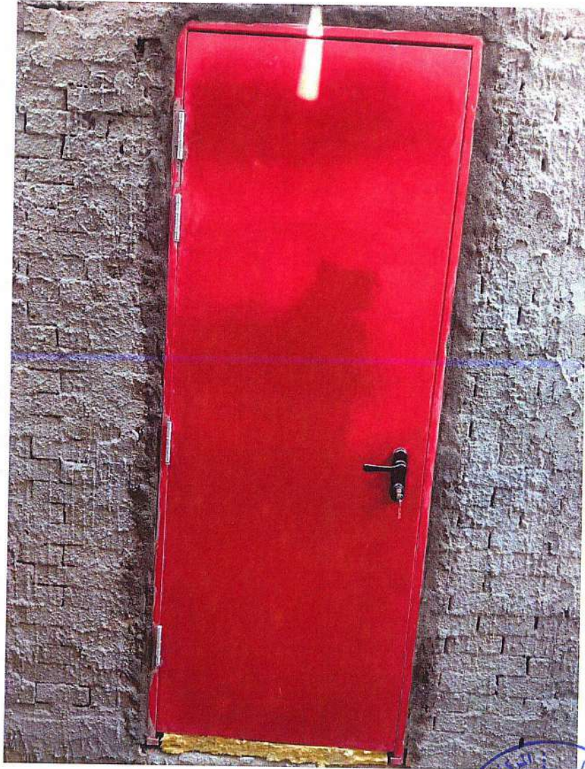
Figure (3): Photo of the exposed face of the door before the test.
