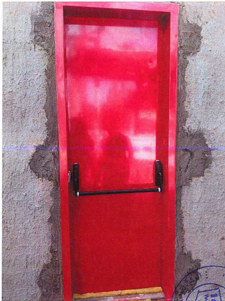
Figure (1): The photo of the unexposed face of the door before the test.
